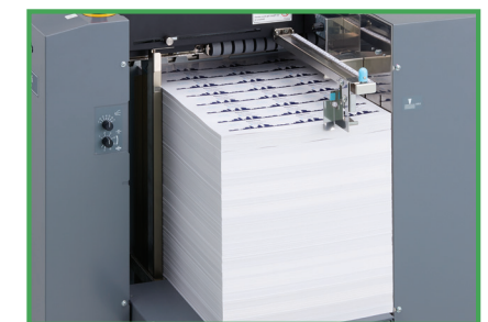
High pile feeder with 8-belt air suction feed system
